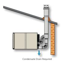
Balanced flue roof outlet (type C32)
