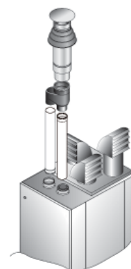
Balanced flue roof outlet (type C32)
