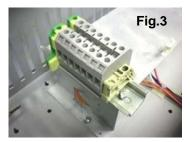
**5:** Certain models, (1.0 metre and 1.5 metre), have two additional orange wires which originally would be connected to the PCB board (see Fig.2). These should be fitted to the new terminal rail as shown in Fig.4. overleaf.
