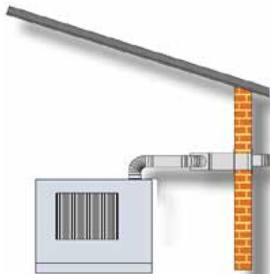
Balanced flue wall outlet (type C12) eliminates expensive roof opening and flashing
