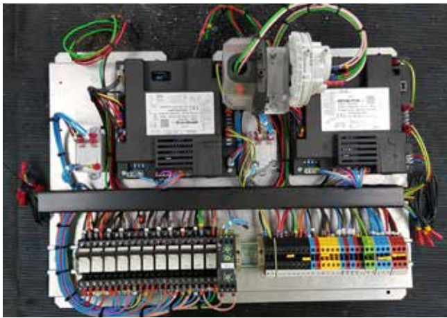
Figure 13 : Control panel assembly located on a removable bracket
