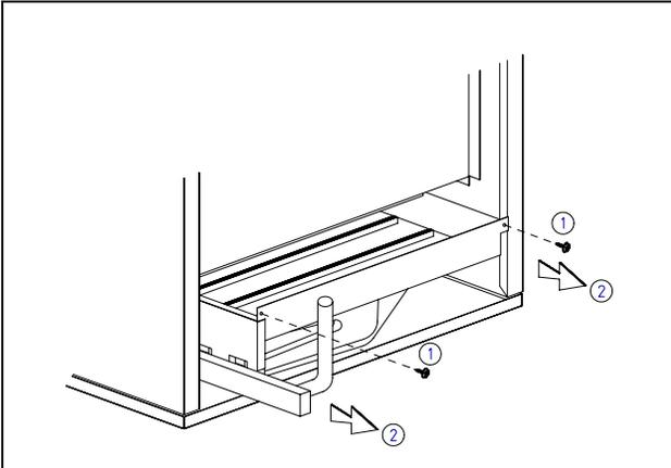
**TO REMOVE BURNER ASSEMBLY:**
