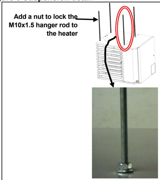
Be sure that the threaded hanger rods are locked to the heater as illustrated. Recommended maximum hanger rod length is 1.8m.
