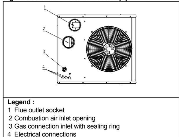
Each heater installed as a type B appliance must be fitted with an individual flue pipe and the combustion air inlet opening must be provided with a protection grill (ask your Reznor distributor for the appropriate protection grill (IP20) (dia130 = PN 02 25094 ). Each heater installed as a type C appliance must be fitted with an individual combustion air/flue pipe system. Only systems specified by the air heater manufacturer may be used.
