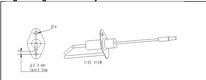
Fig. 10b : Fitting the ignitor
