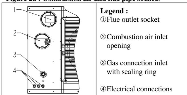
Each heater installed as a type B appliance must be fitted with an individual flue pipe and the combustion air inlet opening must be provided with a protection grill (ask your AmbiRad distributor for the appropriate protection grill (IP20) (1). Each heater installed as a type C appliance must be fitted with an individual combustion air/flue pipe system. Only systems specified by the air heater manufacturer mat be used.
