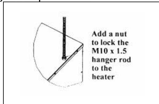
**Be sure that the threaded hanger rods are locked to the heater as illustrated. Recommended maximum hanger rod length is 1.8m.**
