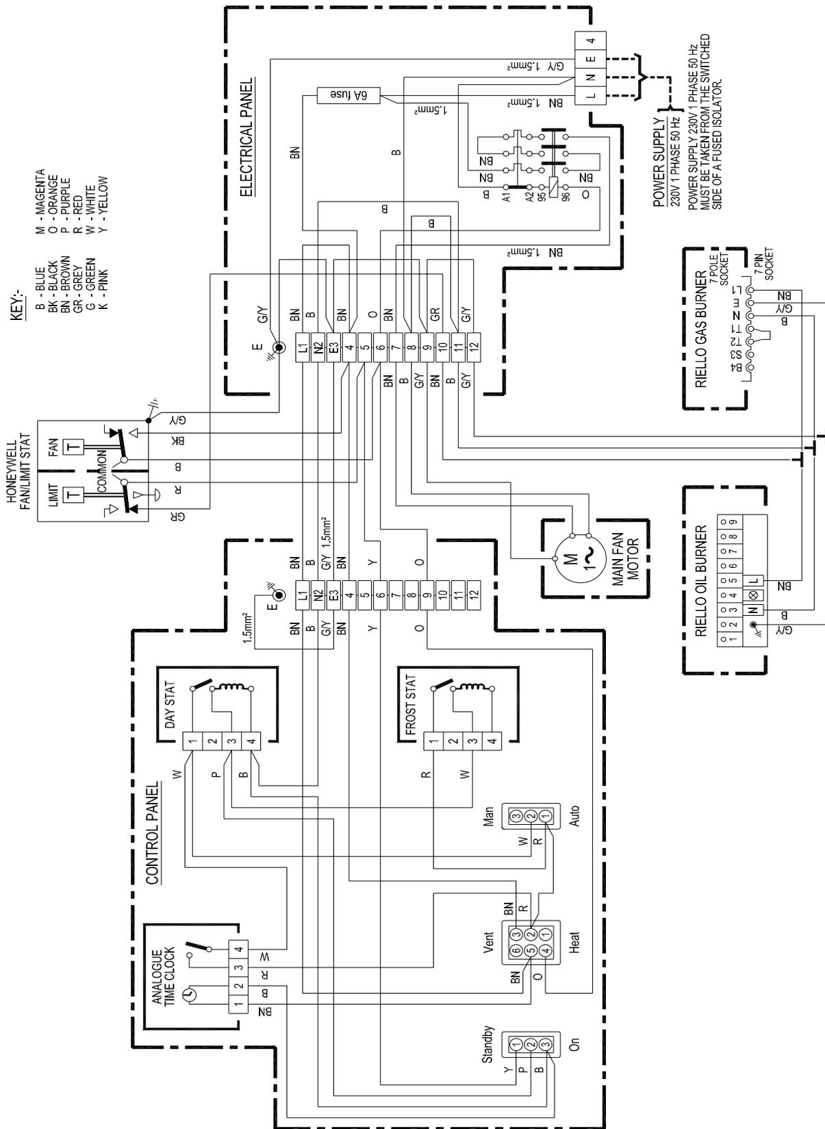
**400-500 Riello ON / OFF Gas or Oil Fired Burner
