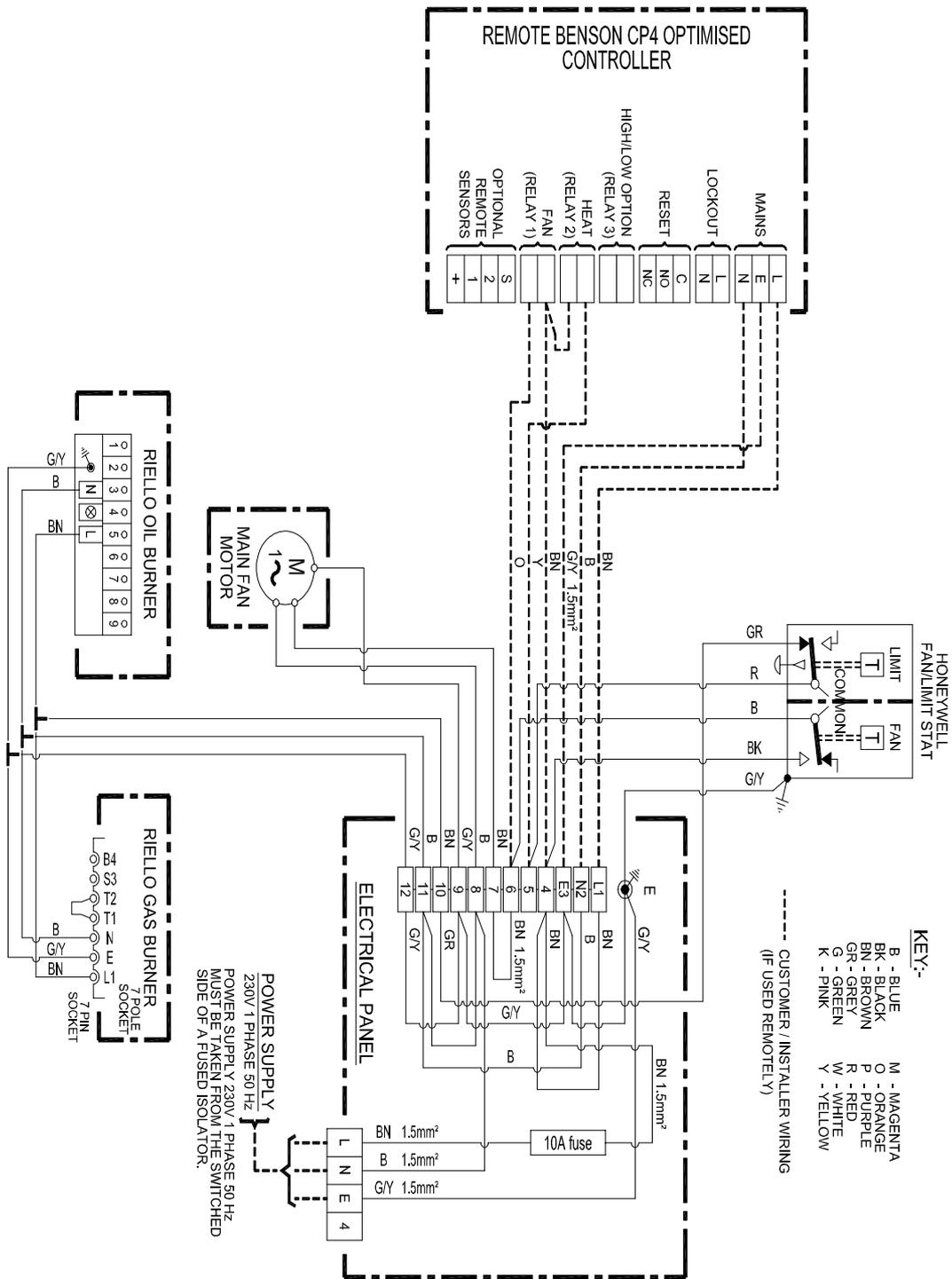
**100-300 Riello ON / OFF Gas or Oil Fired Burner
