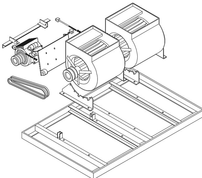
Traces of surplus lubricants spreading from the bearings should also be cleaned away. Where motors are fitted with grease nipples bearings should be lubricated with the correct grade of lubricant. Motors which do not have grease nipples feature sealed bearings which are lubricated during manufacture for their life.
