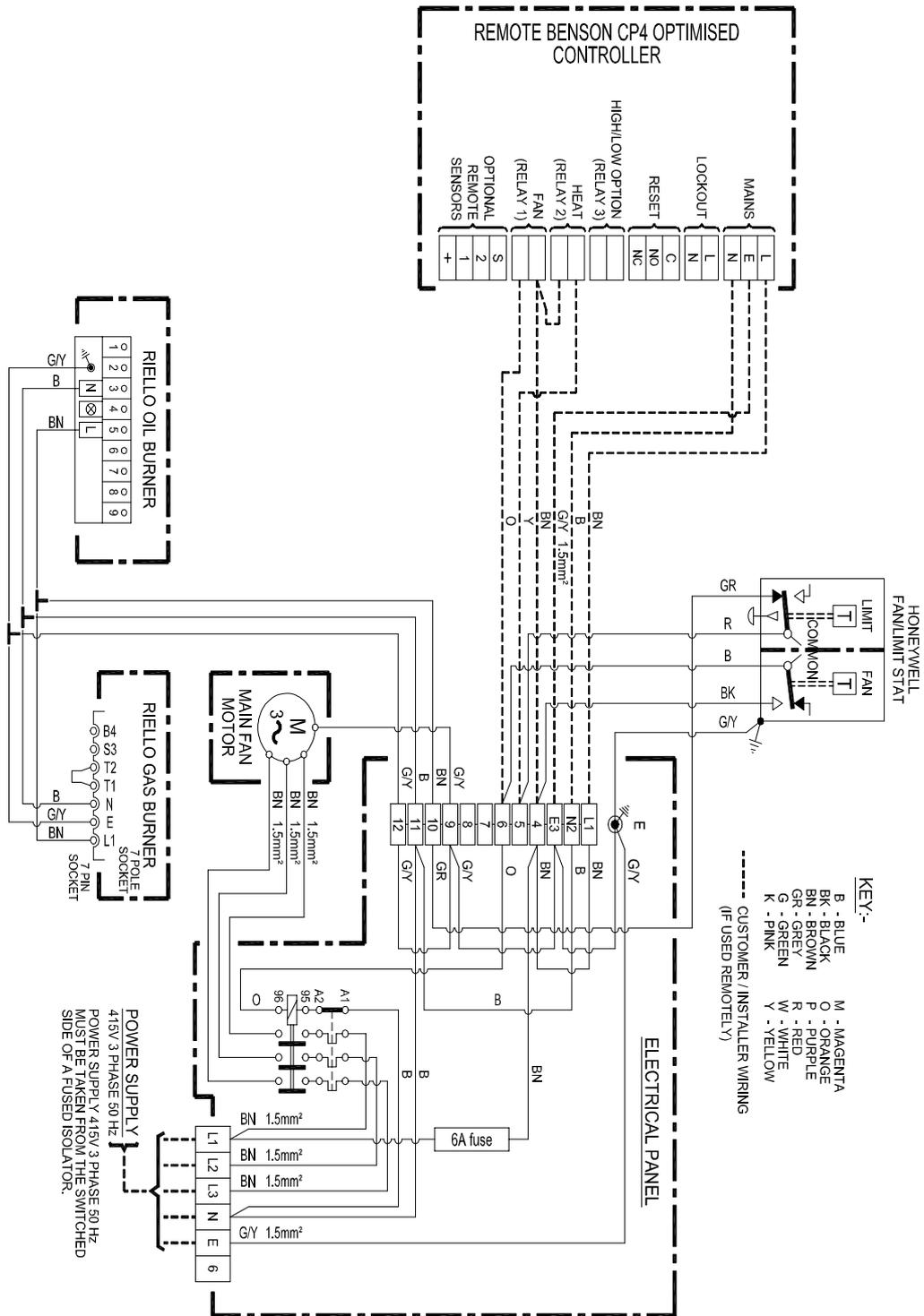
**200 – 1000 Riello ON/OFF Gas or Oil Fired Burner
