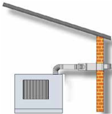
Balanced flue wall outlet (type C13) eliminates expensive roof opening and flashing
