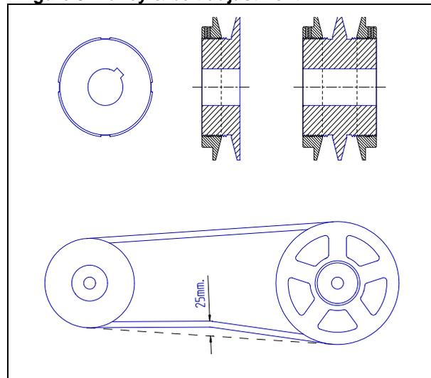
8.4.4 If the amount of adjustment is not achieved with the pulleys fitted, it will be necessary to change the driven pulley fitted on the blower and possibly the size of the drive v belt. **After adjustment ensure the motor load rating is not exceeded!**
