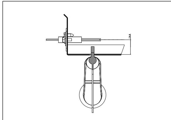
**Figure 18. COMPONENT PARTS LOCATION THERMOELECTRIC BURNER CONTROLS**
