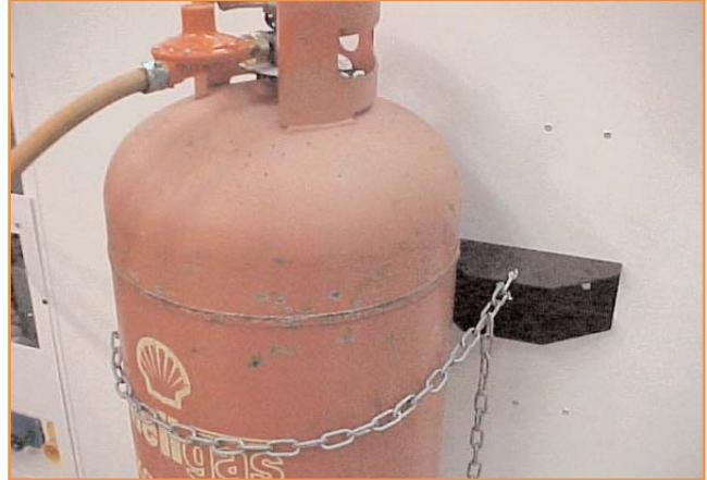
Locate the gas cylinder in the arc of the bracket on the rear of the unit. Pass the chain around the cylinder and through the keyhole slot to ensure that the cylinder is attached to the heater during operation.
