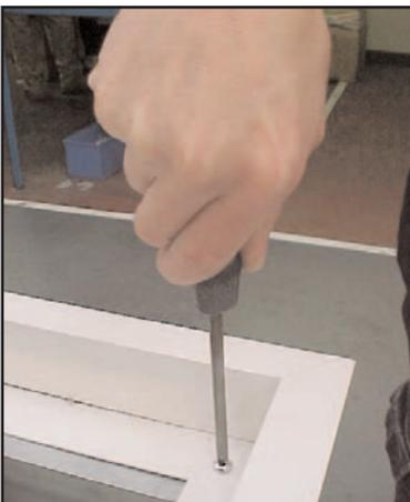
Using the screws provided fit the outer frame to the top of the product case at each corner.
