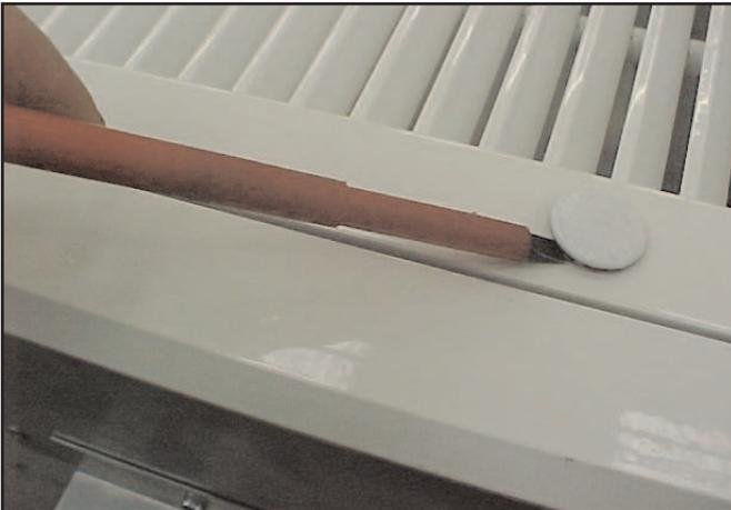
To remove grille from the casing, gently remove the grommets from the inner grille frame.
