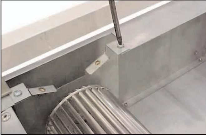
Remove fastening holding rotor support bracket
