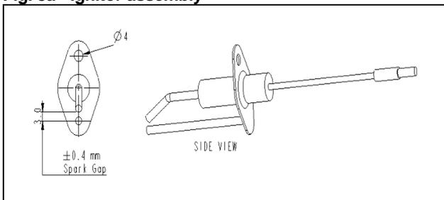
Fig. 8b : Fitting the ignitor
