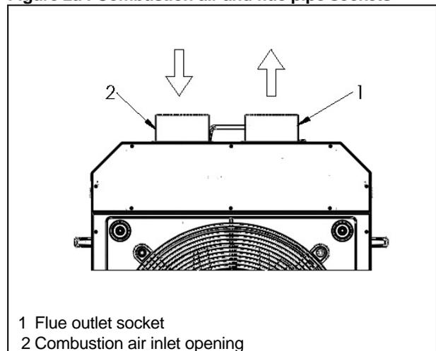
Each heater installed must be fitted with an individual combustion air/flue pipe system. Only systems specified by the air heater manufacturer may be used. Common flue and combustion air systems must not be used.
