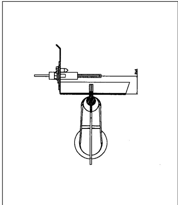
9.14 Figure 13 shows the approximate flame pattern of the ignition burner and its relationship to the flame proving thermocouple.
