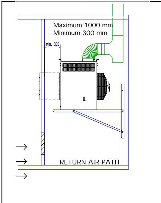
A return air grille must be provided to ensure that an unobstructed path for recirculation; air back to the air heater is maintained, this is to ensure that a negative pressure cannot develop within the space where the air heater is installed.
