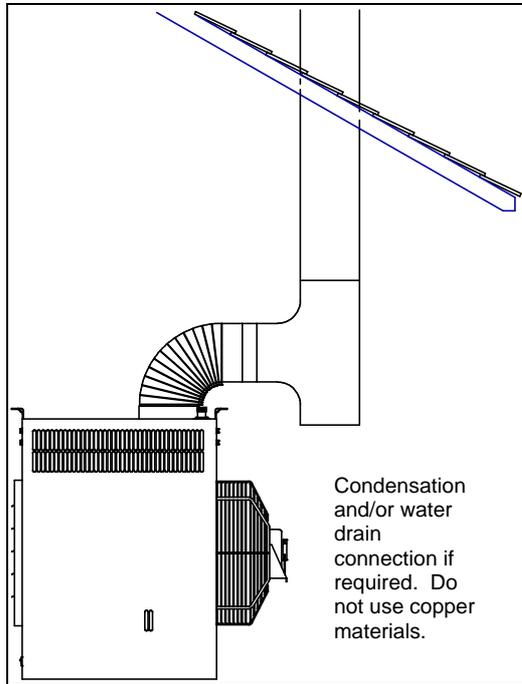
Figure 5. HORIZONTAL FLUE CRITERIA
