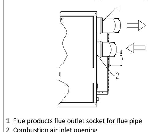
**Table 6 Combustion air inlet & flue pipe requirements**
